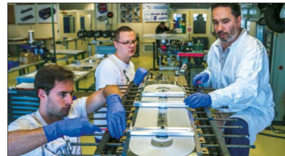
Fig. 2. Left: winding of the enhanced racetrack model coil (RMC) for FCC-hh 16 T magnets with Nb 3 Sn superconducting cable at CERN. Right: A 1 m-long prototype of the FCC-ee dipole magnet. The proposed design considerably reduces the power consumption and the total amount of material required. For example, a machine three times longer than LEP will only require around 35% more steel.
