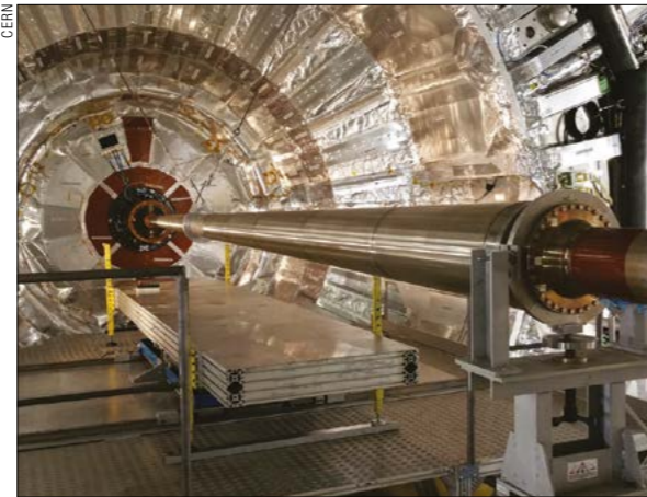
Fig. 2. The central beam pipe of CMS is entirely coated with NEG materials on the inside to ensure the lowest possible beam-gas background to the detector and suppress electron-cloud development.
